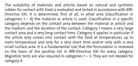
Gaskets for pipes, like novapress® UNIVERSAL, are classified in category 4 by definition. See BfR-Directive XXI (category 4, point 2.4.1 Definition) in this context too. This means that no components representing a hazard to health can be expected to migrate to food if the material is used properly.
