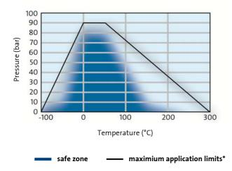
The temperature and pressure recommendations in the graphs apply to gaskets with a thickness of 2.0 mm and raised face flanges. Higher stresses are possible when thinner gaskets are used! The information provided must therefore be considered as estimates that are on the safe side rather than as specific operational limits.
